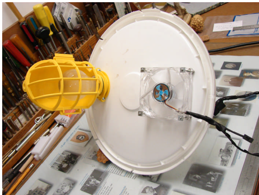
Cooling Fan and Trouble Light Lid Installation Completed
