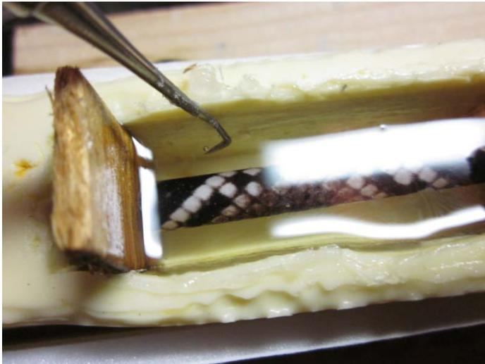
That's it! I move my molds out into the sun to cure. Now, about the petroleum jelly. PR won't stick to it so when you de- mold the blanks you can simply pull off the wood pieces, no saw required.
