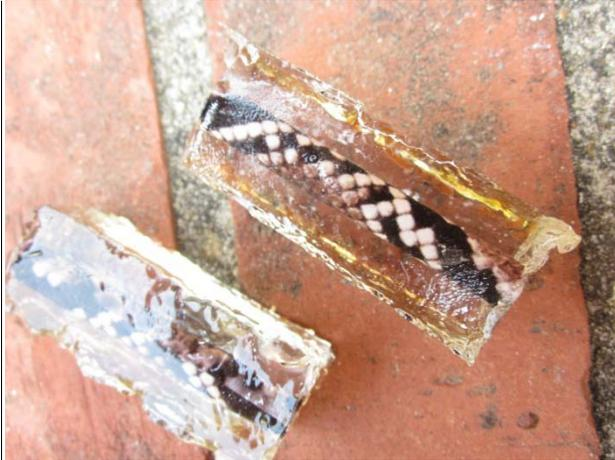
And another example blank (I whipped extra air into the resin to see how well this would work):
