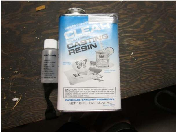
Pour enough resin to fill your mold into a cup and mix in MEKP. I use 3 drops per ounce of resin.
