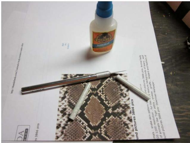
Cut the label to just a bit wider than the tube and apply a line of medium CA on one of the longer edges. Set the tube in the line of glue.
