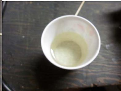
To remove any bubbles you stirred into the resin, hold the cup on the vibrating table with the motor turned on.
