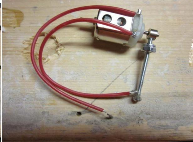
Now that the glue has cooled, mount the motor on one end of the board. You can use tape, but a better way is to screw a thin board into the 2x4 holding the motor in place.
