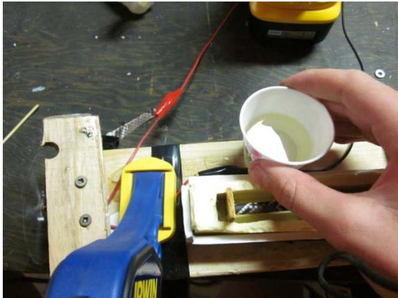
It's (finally) time to pour. Pinch the cup to make a pour spout and pour a thin line of resin into the mold.
