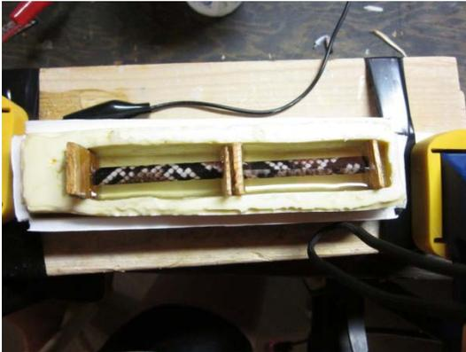
Using a dental pick, start to move the larger bubbles away from the tube with the motor still running.
