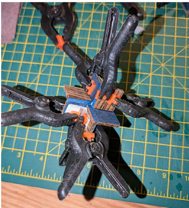
Place a small bracket on the opposite side of the layer and repeat with clamps. This might seem a little excessive but can make a big difference in keeping the halves square whilst the glue sets.
