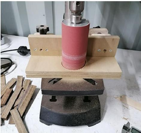
Because my bandsaw tends to drift a little I then run the strips through a thicknesser, it's very basic but does the job well. This also removes any saw marks from the faces of the strips but more importantly guarantees each strip is exactly the same thickness. If you are confident your bandsaw is set up and cuts true there is no need for this stage.
