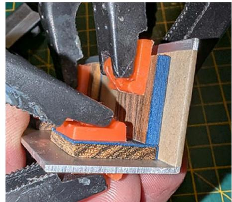
Once the glue has set remove the L segments from the bracket, sand off any excess glue or paper fragments with fine sandpaper and check for any misalignments.
