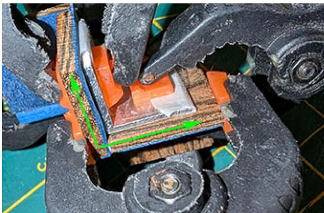
I use small aluminium brackets covered in baking paper to ensure the two halves are absolutely square. Remember to remove any excess glue from between the tiles after gluing, then place in the little bracket and clamp it on both sides.
