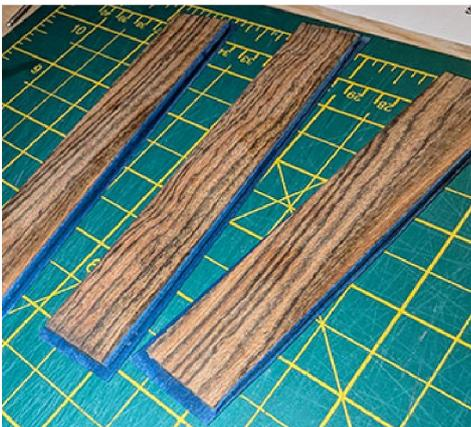
Then bond veneer to the face of the strips, again with the grain of the veneer running in the same direction as the strip of timber. I usually make the veneer slightly larger than the strip taking care to remove any excess glue with a damp cloth before clamping the veneer to the strip. This will guarantee a good L edge/face. When the glue has set remove any excess veneer with a sharp craft knife.
