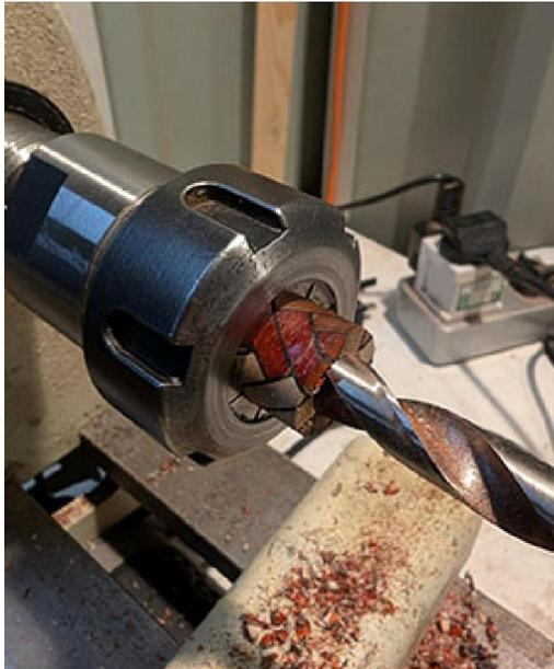
The reason I turn down the blank to just under 20mm is so I can mount it in a collet chuck, this keeps even pressure all around the blank whilst drilling. It also means I have less to remove from the blank once it's mounted on a tube or core and ready to be turned to shape. When drilling the blank take short steps removing the bit completely from the blank between each plunge, try and avoid getting too much heat in the blank as well as this can affect the integrity of the blank.
