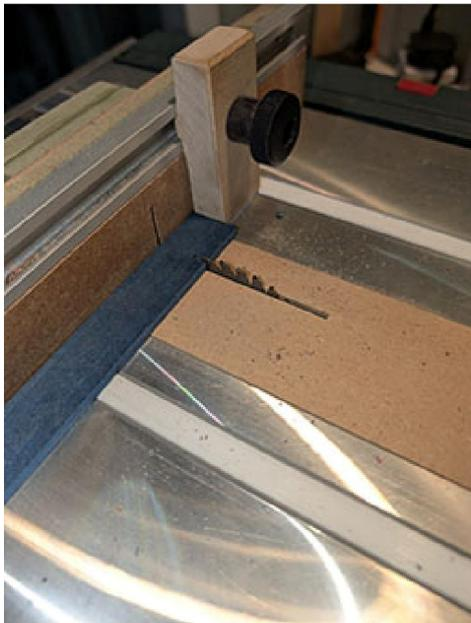
Finally I cut the strips in to square tiles, I have a purpose built crosscut sled for my mini table saw that gives me fairly accurate square cuts. Remember to measure the width of the strips as this will give you the size to cut for your tiles and allow for the width of your saw blade cut as well.
