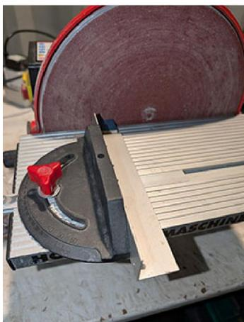
I have a simple jig on my disc sander that allows me to re square the tiles. Unfortunately reworking tiles like this means some tiles end up a little narrower, but are still perfectly usable as long the edges, faces and angles that will end up on inside of the blank are true.
