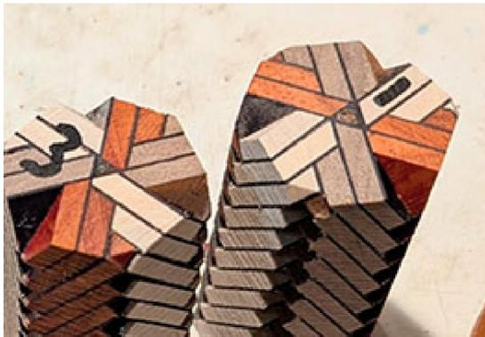
At this stage it's quite easy to find the centre of the blank as it will be highlighted by the veneer. I use a small centre drill bit and drill in just enough so I can then locate the blank between centres on my lathe.
