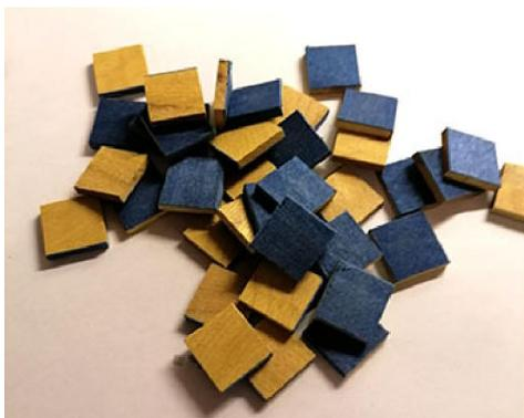
Using the sizes and thickness I've discussed, if I make 72 tiles, using 6 tiles in each layer and therefore 12 layers, I can normally get a finished blank to be 70mm (2.5 to 3 inch) long once the ends have been trimmed from the blank. Obviously if you need a longer blank than this then more layers will need to be added.
