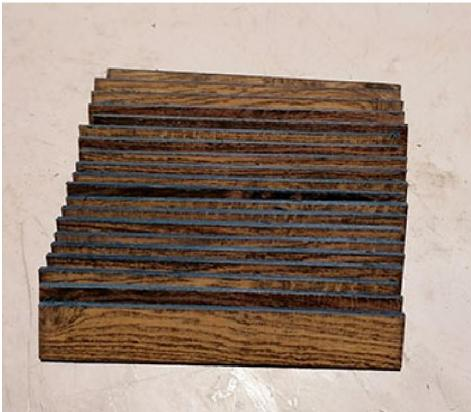
I then ran the blocks through my bandsaw cutting through the veneered face to give strips approximately 5mm thick. Seems obvious but is the easiest way to get veneer on the thin face of what will eventually be a tile.
