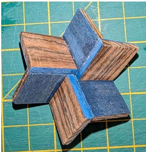
A completed layer can be seen here and multiple layers of the same thing gives an impression of highlighted or accented rectangles in the final blank.
