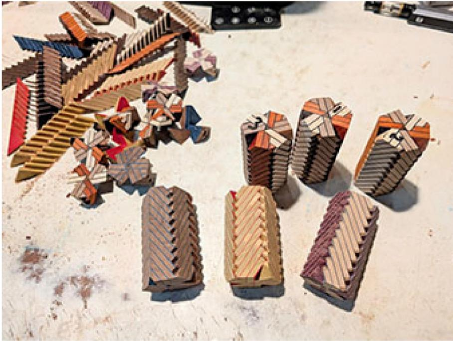
Once I'm happy that everything is truly bonded and stable I remove what I call the wings from the blank and square the ends. I then remove any extreme edges from the length of the blank on a disk sander.
