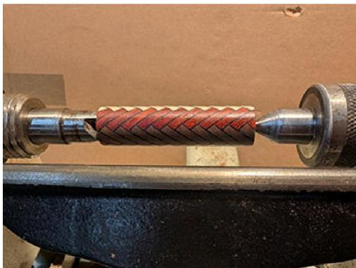
I use a prong drive and live centre and turn the blank down to just under 20mm, if you are using pen jaws on your lathe or a pen vice and pillar drill for drilling the blank I'd suggest turning down to around 30 mm. This will keep enough integrity in the blank and avoid any blow out whilst drilling.
