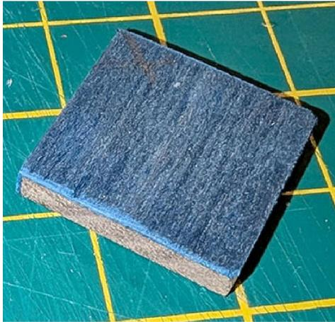
Each tile has veneer on one face and an adjacent side forming an L shape around the tile. It is important that each tile is same thickness. I usually make the tiles around 3.5mm to 4.5mm (1/8 to 3/16 inch) thick, anything larger than 6mm (1/4 inch) the tiles may lose their rectangular appearance when the final blank is turned down, this is important especially if you intend to make a thin pen with the blank.
