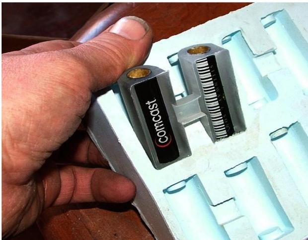
The tubes should be installed on the stoppers closest to the center of the mold first. Once seated, gently pull on the outside wall of the mold to allow the tubes to be installed. Gently release the mold wall, sliding the outside stoppers into the tube. This will help avoid any stopper damage caused by sharp tube edges.
