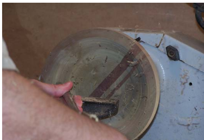
Figure 14: Turn the inside of the bowl first, being careful to only remove enough wood to even out the rings.
