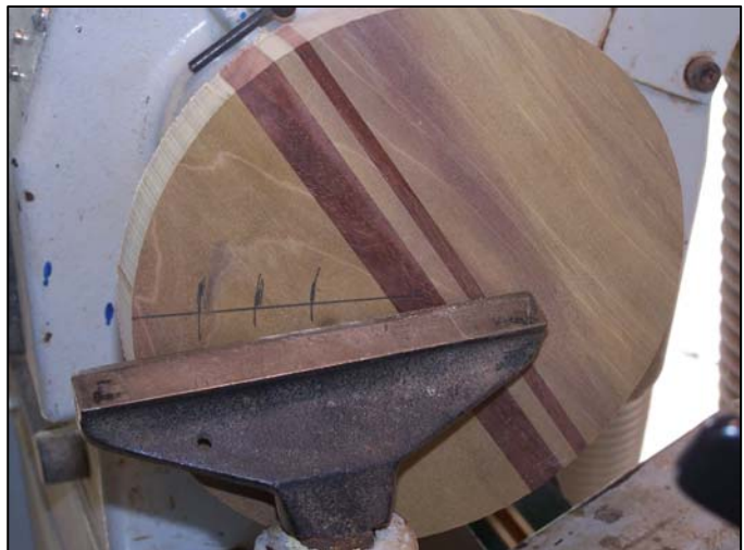
Figure 9: Draw a line and make "tick" marks along the bowl. Then rotate the disk to create a full circle at each mark
