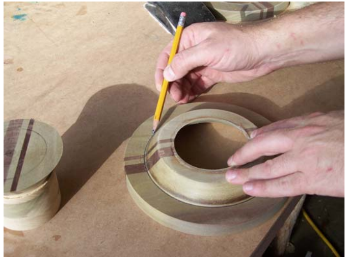
Figure 12: Reverse stack the pieces, and carefully align them. Then trace the pattern from one to the other.
