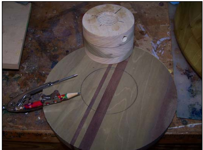
Figure7: Mark the center of the blank with a compass just slightly larger than your waste block. This will help align the block when you glue it to your bowl blank
