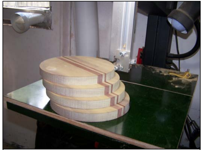
Figure 6: Four “bowl blanks” cut from the scrap. Using the circle cutting jig makes truing the blanks much easier once they are mounted on the lathe.
