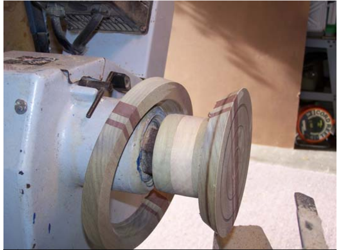
Figure 11: The first ring falls back behind the blank. Stop the lathe and remove the faceplate and then the ring. Repeat for each ring. Note the angle of the parting cut.
