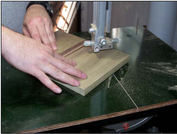
Figure 5: A circle-cutting jig makes it easy to cut the blanks round. But you can free-hand it if you are comfortable with that.
