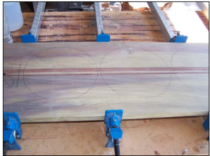
Figure 4: Using the template, we get four blanks out of this one board
