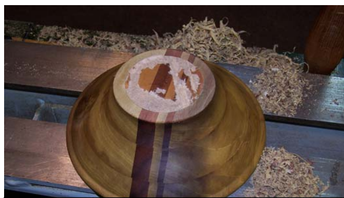
Figure 15: Break apart your paper bag glue-up with a mallet and sharp chisel. You get a nice clean break with only some paper residue (no split wood or screw holes) that's very easy to sand or turn away.
