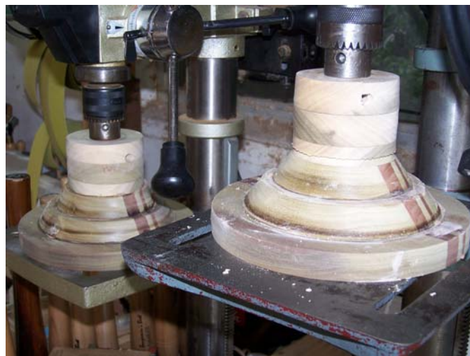
Figure 13: Once glued-up, I use my drill press to clamp the rings together under pressure.
