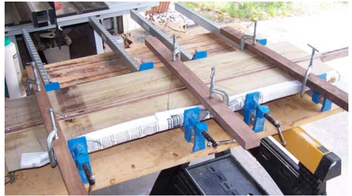
Figure 2: Glue the strips in your preferred layout. Use plenty of clamps and cawls to ensure a good bond
