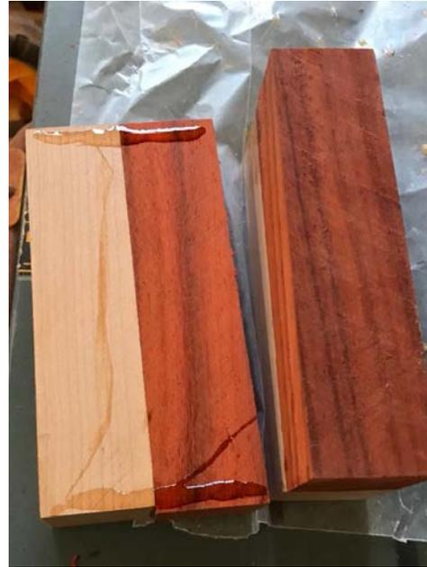
Glue waste plywood on ends to reinforce the blanks, turn, sand and finish inside of the ornaments. Cutoff glued ends so that the four pieces can be separated.
