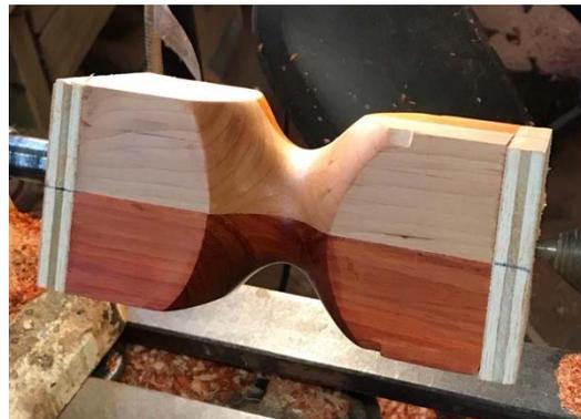
Cut odd the ends and reverse the the pieces so that the turned section is inside and reglue the blanks.
