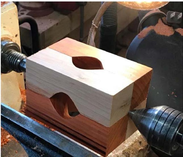
Turn the outside of the blank, cut off end, sand and finish.
